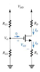
4. Design the circuit shown below so that the transistor operates in saturation with  $V_D$  biased 1 V from the edge of the triode region, with  $I_D = 1$  mA and  $V_D = 3$  V for each of the following two devices (use a 10- $\mu$ A current in the voltage divider):
