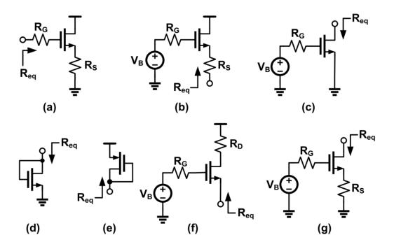
2. Using the results from Problem 1, determine the equivalent impedance for the configurations shown below. You may assume all transistors are biased in saturation region and  $r_{ds} \neq \infty$
