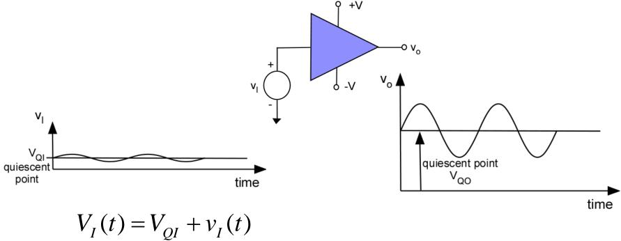
$$V_{I}(t) = V_{QI} + V_{I}(t)$$
