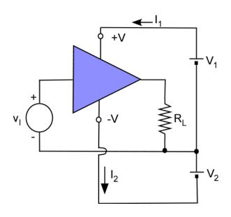
$$P_{DC} = V_1 I_1 + V_2 I_2$$
