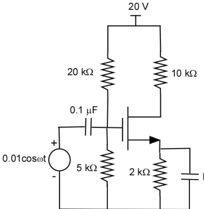
$$V_{GQ} = V_{DD} \frac{R_2}{R_1 + R_2} = \frac{20 \times 5}{25} = 4 \text{ V}$$
