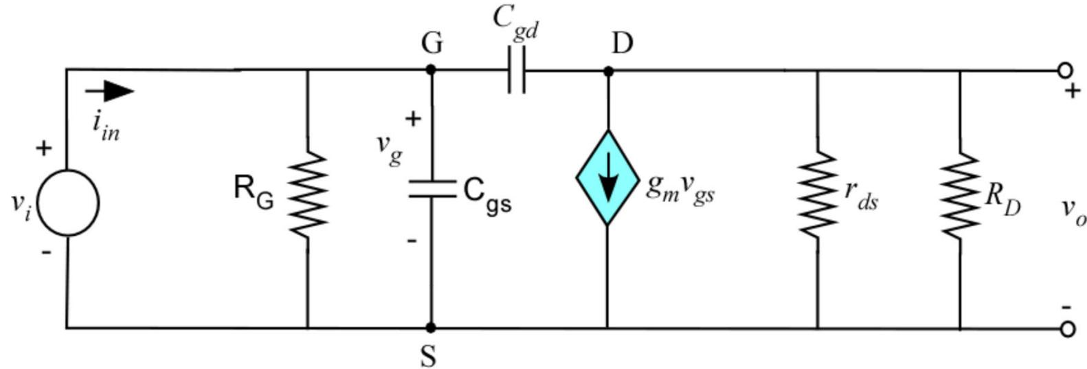
$$\text{If } R_i = 0, \quad f_{3dB} = \frac{1}{2\pi C_{gd} R_D} \quad r_{ds} = \frac{|V_A|}{I_D} = \frac{20}{1.516} = 13 \text{ k}\Omega$$
