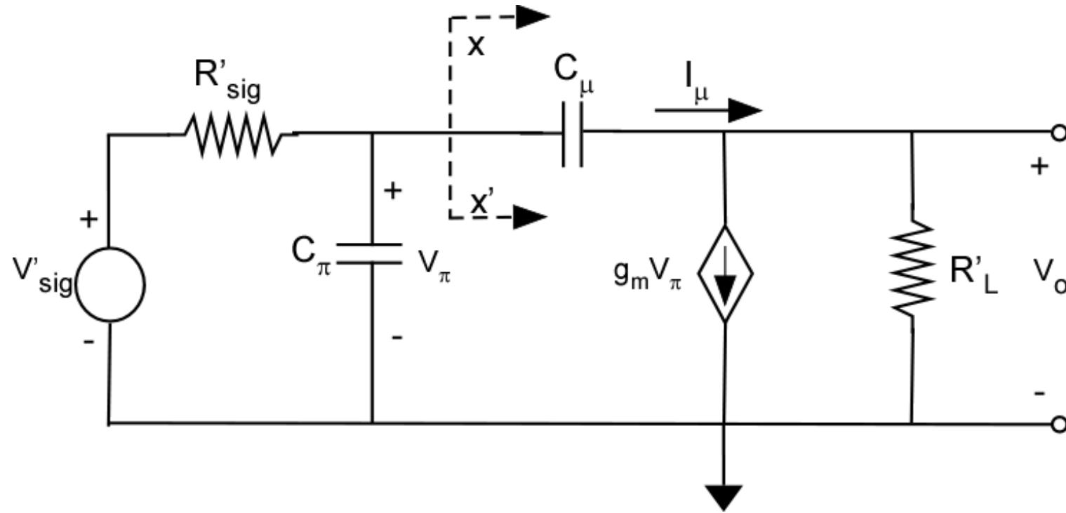
The left hand side of the circuit at XX' knows the existence of  $C_\mu$  only through the current  $I_\mu \rightarrow$  replace  $C_\mu$  with  $C_{eq}$  from base to ground
