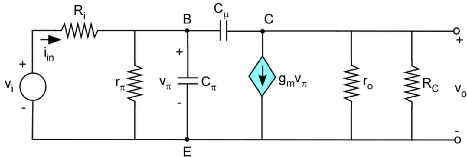
$$\frac{v_o}{v_i} = -\frac{G_s R'_C (g_m - sC_\mu)}{G_i + g_\pi + s[C_\pi + C_\mu] + sC_\mu R'_C [G_i + g_\pi] + sC_\mu g_m R'_C + s^2 C_\mu C_\pi R'_C}$$
