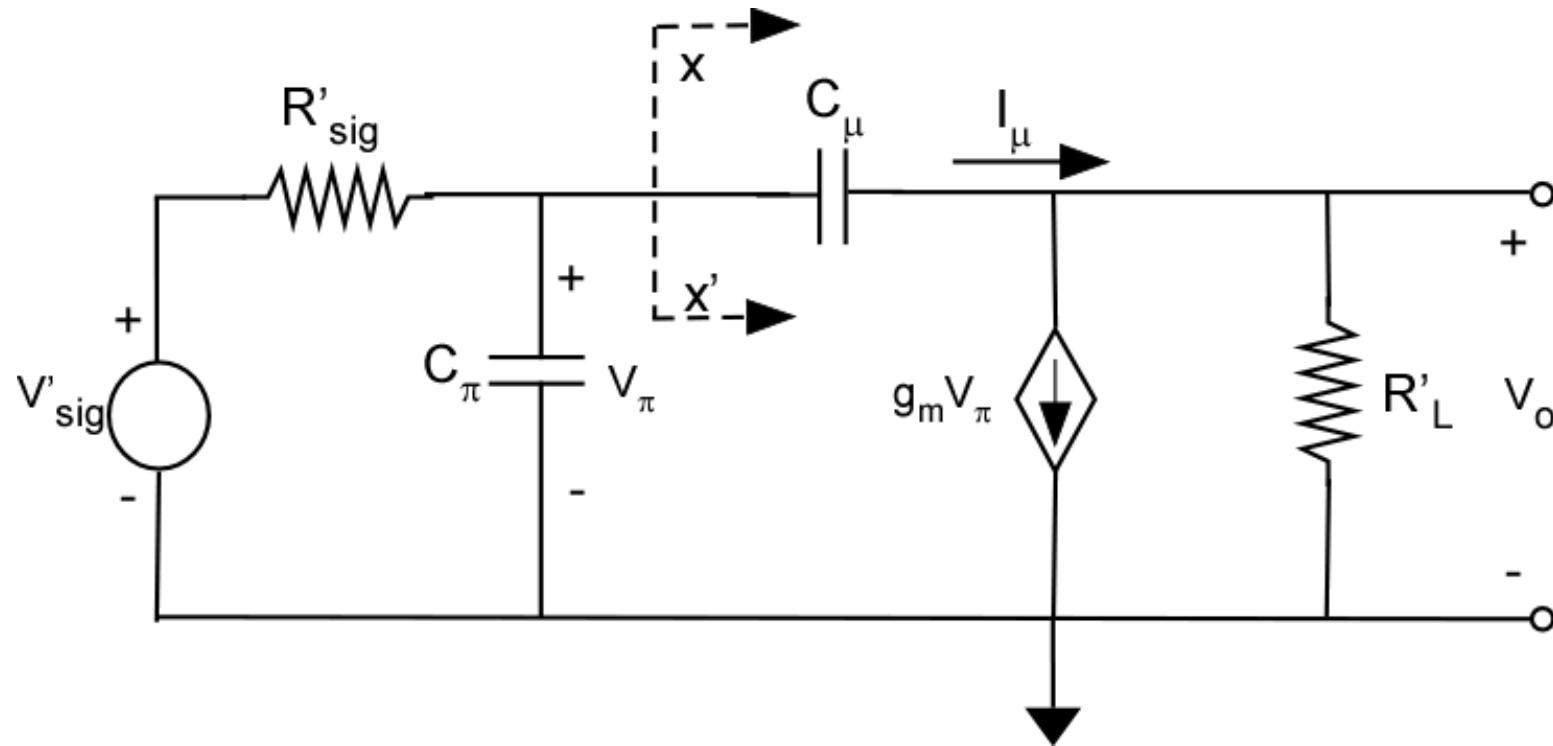
$$V'_{sig} = V_{sig} \cdot \frac{R_B}{R_B + R_{sig}} \cdot \frac{r_\pi}{r_\pi + r_x + (R_{sig} \parallel R_B)}$$
