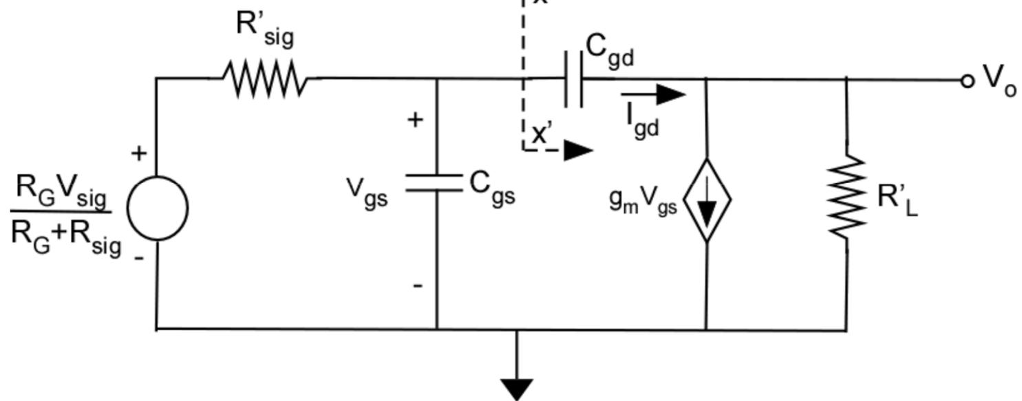
$$I_{gd} = sC_{gd} (V_{gs} - V_o) = sC_{gd} [V_{gs} - (-g_m R'_L V_{gs})]$$
