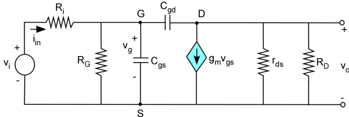
$$G_i = \frac{1}{R_i} \quad G_D = \frac{1}{R_D} \quad G_g = \frac{1}{R_g} \quad g_{ds} = \frac{1}{r_{ds}} \quad R'_D = R_D \parallel r_{ds} = \frac{1}{G_D + g_{ds}}$$
