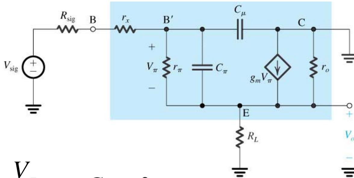
$$g_m V_\pi + \frac{V_\pi}{r_\pi} + s_Z C_\pi = 0$$
