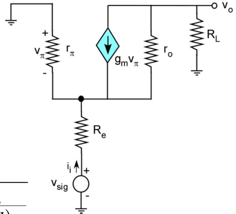
$$R_{in} = \frac{r_o + R_L}{1 + \frac{r_o}{r_e} + \frac{R_L}{(\beta + 1)r_e}}$$
