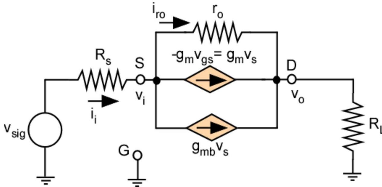
$$i_i = (g_m + g_{mb})v_i + i_{ro} \quad \text{with } v_i = v_s$$
