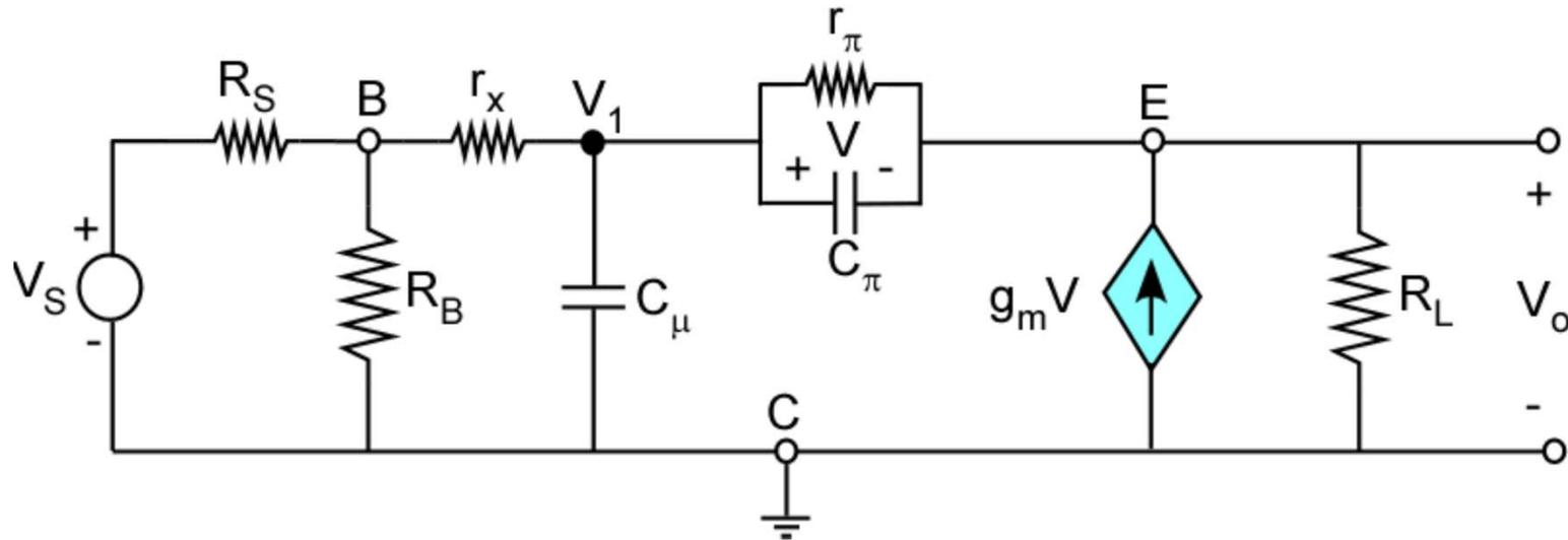
$$A'_v(s) = \frac{g_m R_L}{1 + g_m R_L} \frac{1 + \frac{sC_\pi}{g_m}}{1 + \frac{sC_\pi R_E}{1 + g_m R_E}}$$
