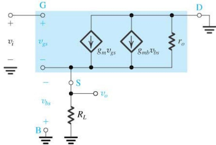
$$R'_L = R_L \parallel r_o \parallel \frac{1}{g_{mb}}$$
