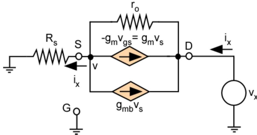
$$v_x = [i_x + (g_m + g_{mb})v]r_o + v \quad \text{with } v = i_x R_s$$
