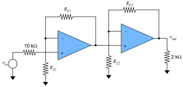
Pick first stage gain 10; second stage gain 20. We must then have:
