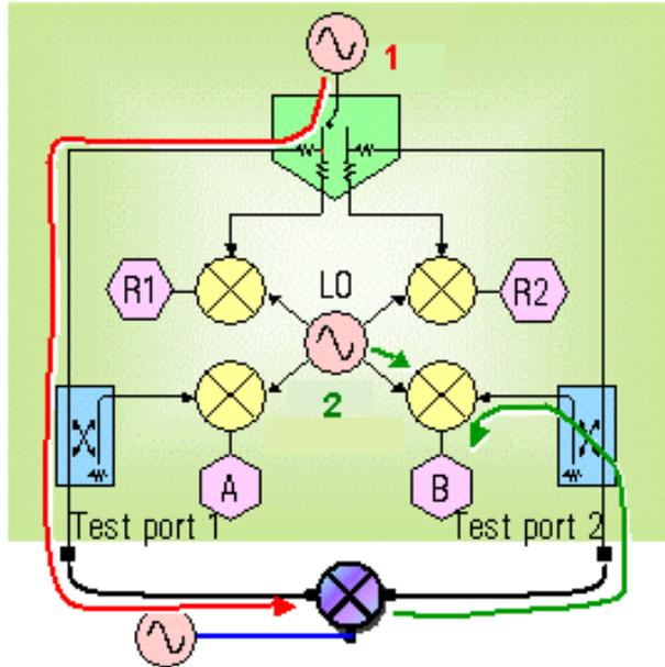
1: Internal source tuned to DUT input
