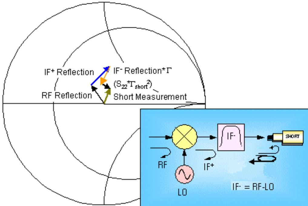
This vector plot shows how the terms combine to make the short measurement. Note in this case that the RF and IF+ reflections are not changed from the open measurement. The IF- reflection has changed phase by 180 degrees, because the  $\Gamma_{\text{Termination}} = -1$  for a short. However, the fourth term ( $S_{22} * \Gamma_{\text{Termination}}^2$ ) is in the same direction as for the open. This is because the term ( $\Gamma_{\text{Load}} = -1$ ) is 1 when squared, just as with the open.
