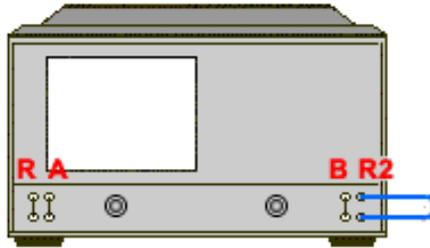
This method balances the delays in the reference and test paths, so that the network analyzer's ratioed transmission measurement does not have a frequency-shift error.
