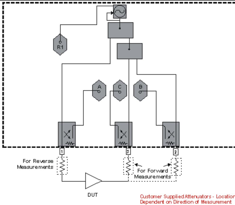
**Diagram: (N338x) Configuration using a Booster Amplifier**
