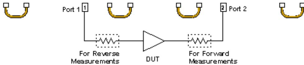
Customer Supplied Attenuator - Location dependent on direction of measurement
