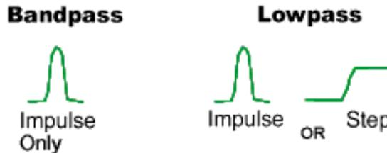
The PNA can present the time domain response as if either an impulse function or a step function stimulated the device under test.
