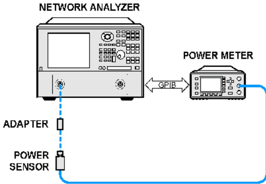
Connecting adapter and cable between sensor and PNA
