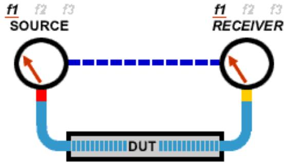
If the analyzer is measuring a long cable, the signal frequency at the end of the cable will lag behind the network analyzer source frequency. If the frequency shift is appreciable compared to the network analyzer's IF detection bandwidth (typically a few kHz), then the measured result will be in error by the rolloff of the IF filter.
