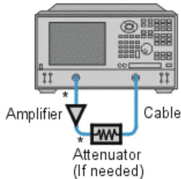
6. Select the analyzer settings for your amplifier under test in order to perform a swept-power gain compression measurement at a chosen frequency. See Gain Compression.
