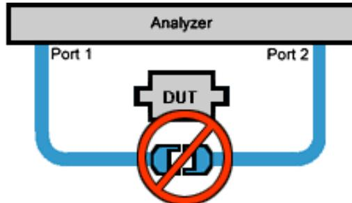
When calibrating for a non-insertable device, you must use an adapter for the thru connection. This adapter is not included in the measurement, and therefore reduces measurement accuracy. If you have a non-insertable device you must choose one of the following methods when making a thru connection during calibration. The methods are listed in order of ascending accuracy (least accurate first):
