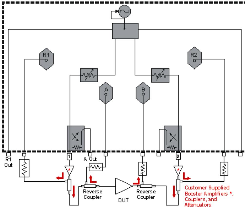
**Diagram: (E835x) Simple Configuration using One Booster Amplifier**
