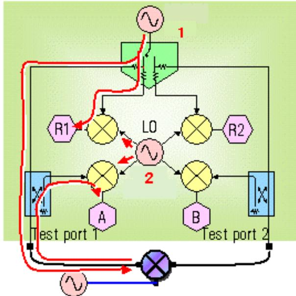
1: Internal source tuned to DUT input
