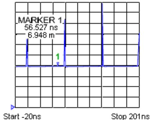
The range is related to the spacing between frequency points in the measured frequency response of the device.
