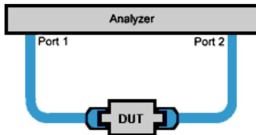
This is the easiest but least accurate method of calibrating for a non-insertable device. "Uncharacterized" means that the thru adapter's electrical delay and loss are not recorded in the analyzer.
