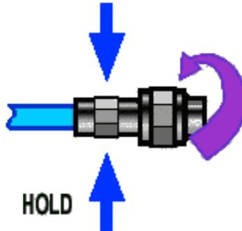
5. Use a torque wrench to make final connection. Tighten until the "break" point of the torque wrench is reached. Do **not** push beyond initial break point. Use additional wrench, if needed, to prevent device body from turning.
