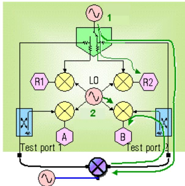
1: Internal source tuned to DUT input
