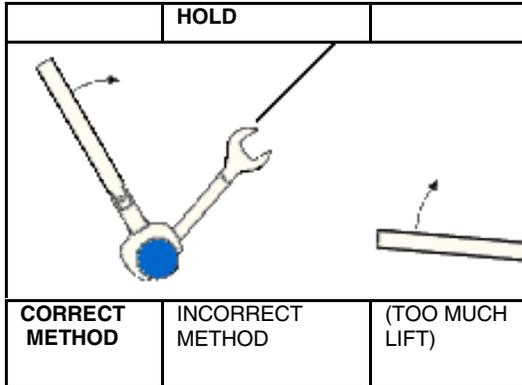
3. Hold torque wrench lightly at the end of handle then apply force perpendicular to the torque wrench handle. Tighten until the "break" point of the torque wrench is reached. Do **not** push beyond initial break point.
