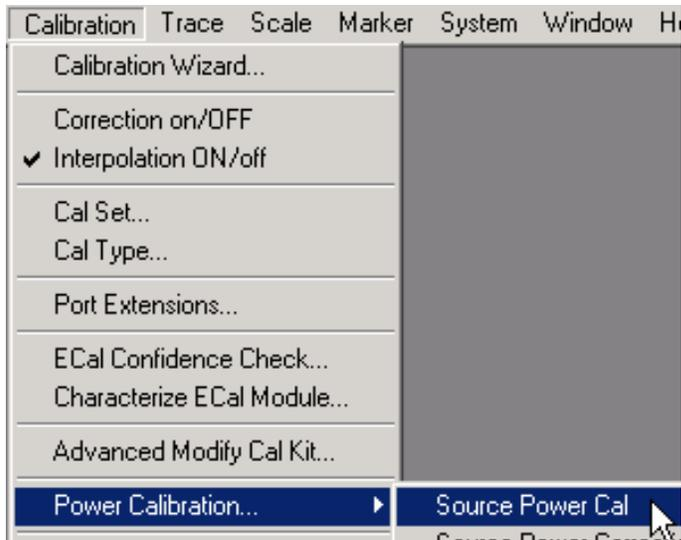
5. Complete the Source Power Cal dialog box (below), including Loss Compensation and Power Sensor Settings, as needed.
