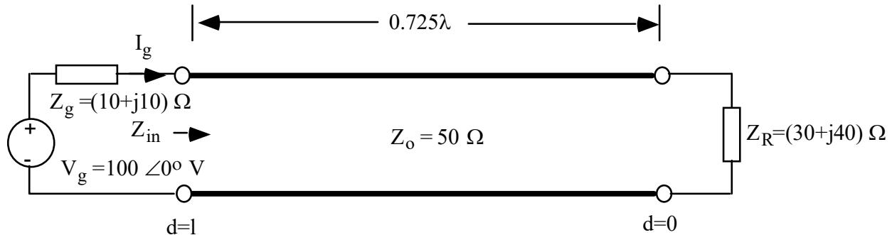
1. Consider the transmission line system shown in the figure above.
