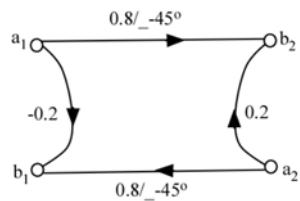
$$S : \begin{bmatrix} -0.2 & 0.8 \angle -45^\circ \\ 0.8 \angle -45^\circ & 0.2 \end{bmatrix}$$
