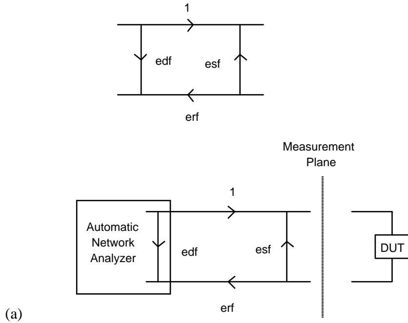
$$(b) S_{11m} = E_{DF} + \frac{E_{RF}S_{11a}}{1 - S_{11a}E_{SF}}$$
