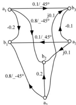
(e) With a  $50 \Omega$  load at port 3, there is no input at  $a_3$ . So, the SFG in (d) simplifies to
