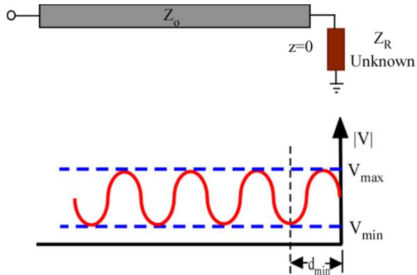
**At minimum,**  $\Gamma(z) = \text{pure real} = -|\Gamma_R|$
