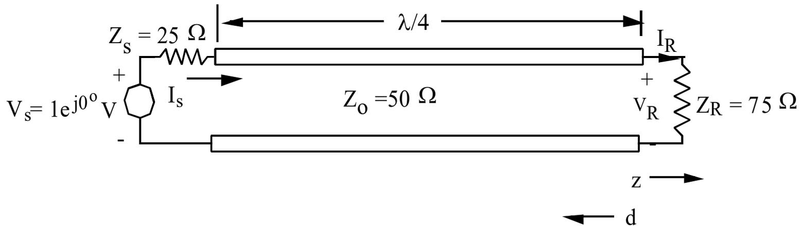
A signal generator having an internal resistance  $Z_s = 25 \Omega$  and an open circuit phasor voltage  $V_s = 1e^{j0}$  volt is connected to a  $50\text{-}\Omega$  lossless transmission line as shown in the above picture. The load impedance is  $Z_R = 75 \Omega$  and the line length is  $\lambda/4$ .
