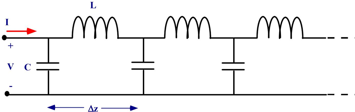
$$-\frac{\partial}{\partial z} \left( \frac{\partial V}{\partial z} \right) = -\frac{\partial^2 V}{\partial z^2} = j\omega L \frac{\partial I}{\partial z} = -j\omega L j\omega C V \quad \Rightarrow \quad \frac{\partial^2 V}{\partial z^2} = -\omega^2 L C V$$
