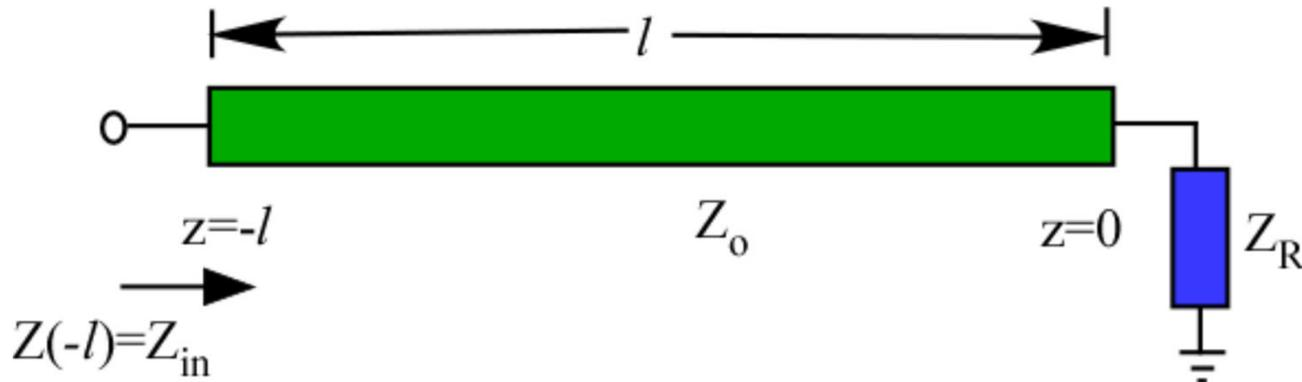
$$Z(z) = \frac{V(z)}{I(z)} = Z_o \left[ \frac{e^{-j\beta z} + \Gamma_R e^{+j\beta z}}{e^{-j\beta z} - \Gamma_R e^{+j\beta z}} \right]$$
