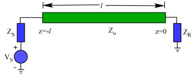
with  $T_S = \left(1 + \frac{Z_S}{Z_o}\right)^{-1} = \frac{Z_o}{Z_S + Z_o}$  and  $\Gamma_S = \frac{Z_S - Z_o}{Z_S + Z_o}$
