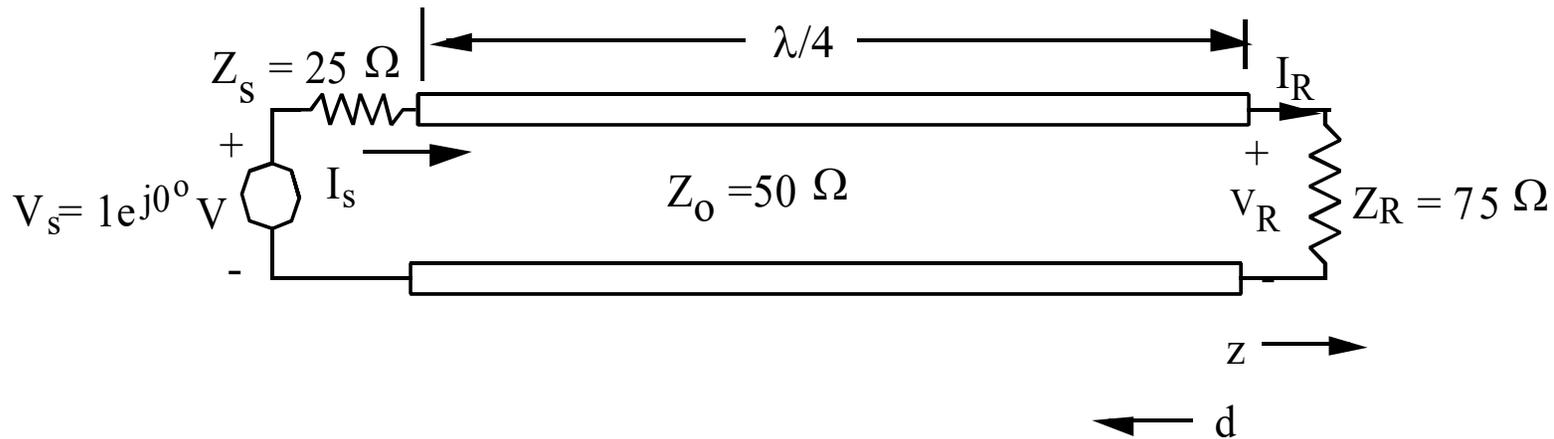
$$V_+ = \frac{T_s V_s e^{-j\beta l}}{1 - \Gamma_R \Gamma_s e^{-2j\beta l}}$$
