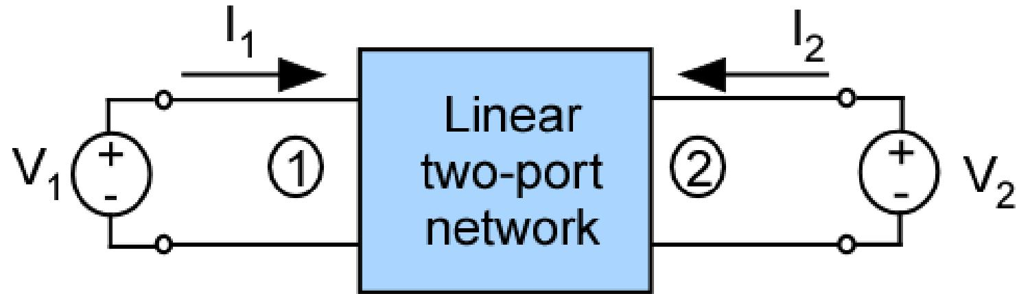
$$I_1 = y_{11}V_1 + y_{12}V_2$$
