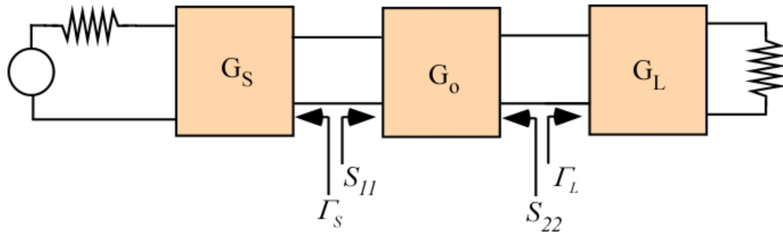
$G_s$  affects the degree of mismatch between the source and the input reflection coefficient of the two-port.
