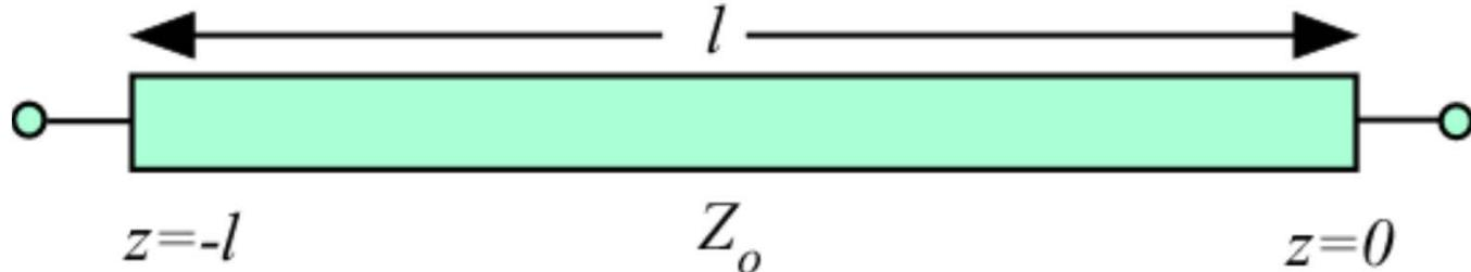
Find the Y-parameters of a lossless transmission line with propagation constant  $\beta$  and characteristic impedance  $Z_o$  (admittance  $Y_o$ )
