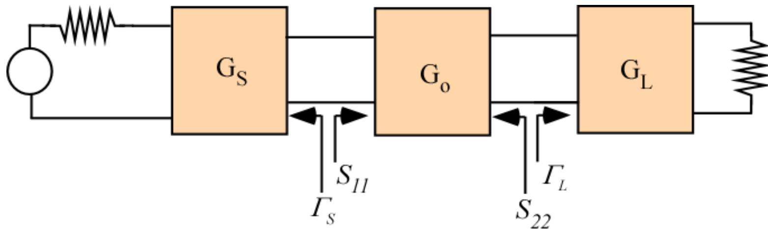
$G_L$  affects the degree of mismatch between the load and the output reflection coefficient of the 2-port.
