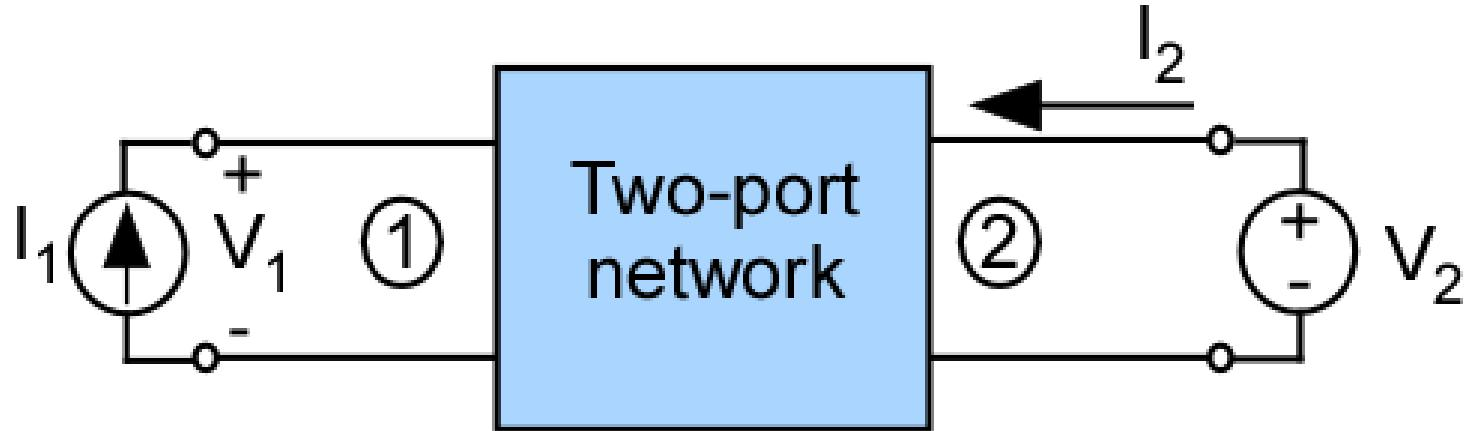
$$V_1 = h_{11}I_1 + h_{12}V_2$$
