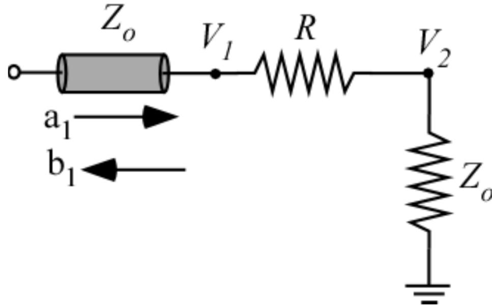
Since  $a_2=0$ , the total voltage in port 2 is:  $V_2 = b_2 \sqrt{Z_o}$
