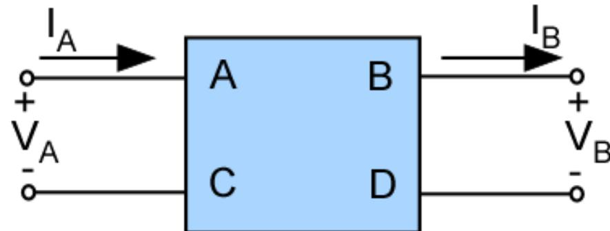
When cascading two-ports, it is best to use ABCD parameters. Put voltage and currents in cascadable form with the input variables in terms of the output variables
