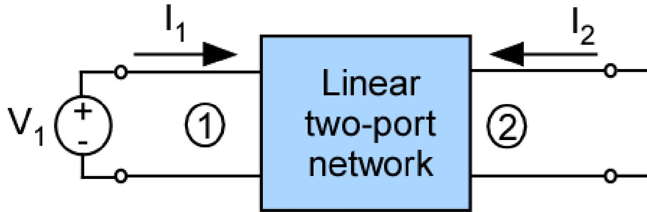
$$y_{11} = \frac{I_1}{V_1} \Big|_{V_2=0}$$
