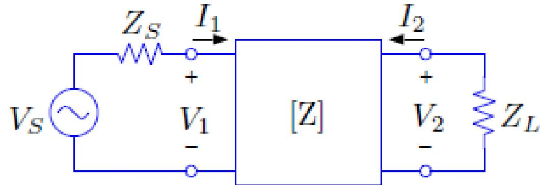
$$G_T = \frac{|Z_{21}|^2 R_L R_S}{|(Z_{11} + Z_S)(Z_{22} + Z_L) - Z_{12}Z_{21}|^2}$$
