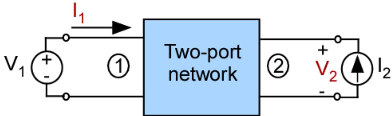
$$I_1 = g_{11}V_1 + g_{12}I_2$$
