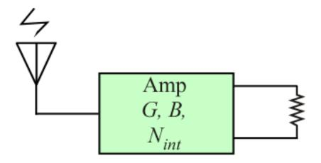
200- $\Omega$  antenna exhibiting an rms noise voltage of 0.1  $\mu V$  with  $B{=}10^4$  Hz
