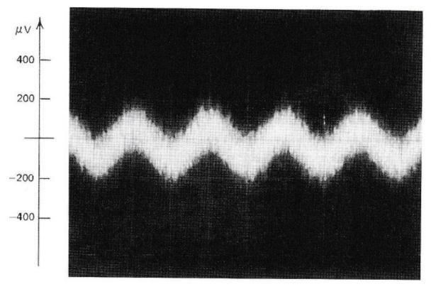
Output voltage waveform for input level comparable to noise level\*
