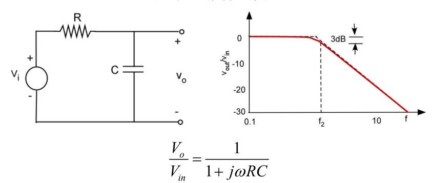
The output voltage drops to 0.707 of its low-frequency value when  $\omega RC = 1$
