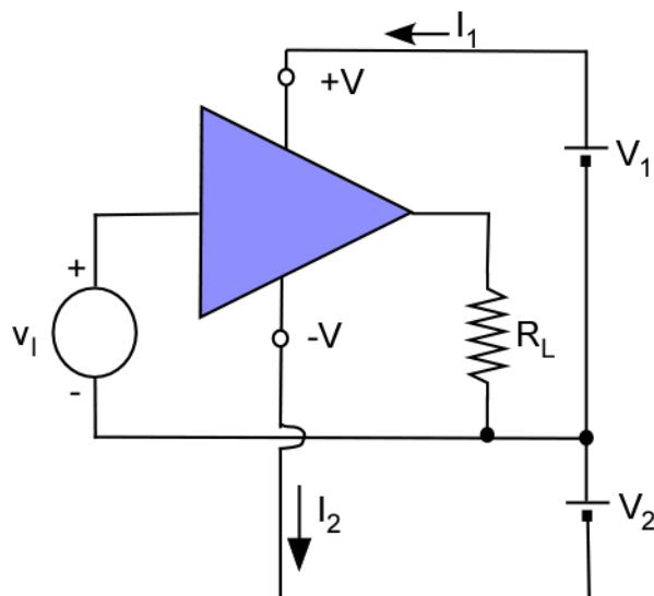
$$P_{DC} = V_1 I_1 + V_2 I_2$$
