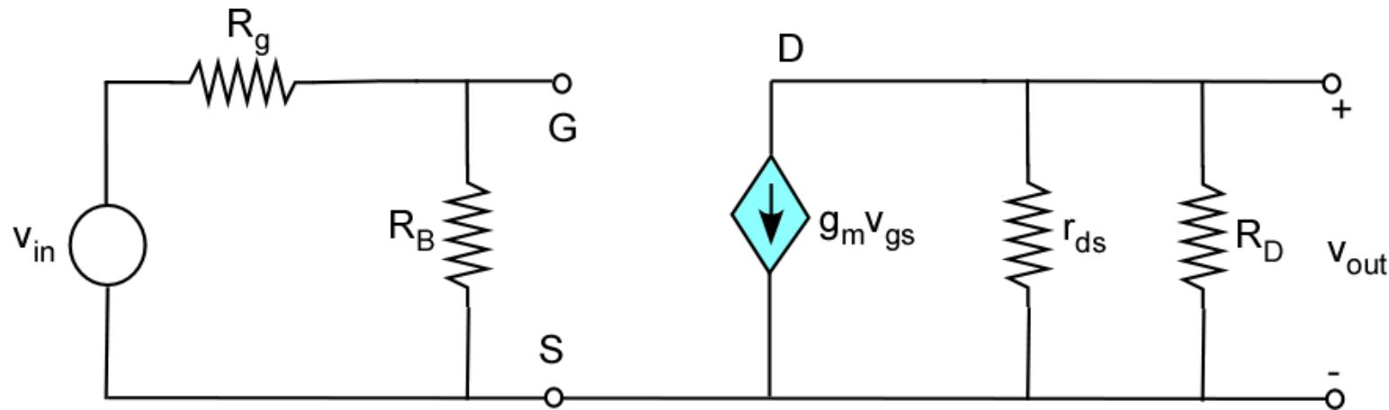
$$A_{MB} = \frac{v_{out}}{v_{in}} = -\frac{R_B}{R_B + R_g} g_m \frac{r_{ds} R_D}{r_{ds} + R_D}$$
