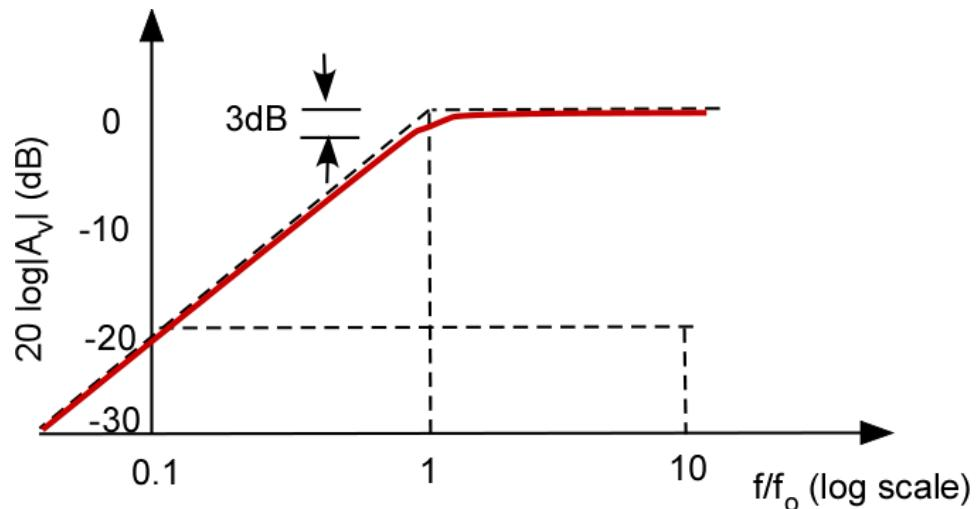
$$V_o = \frac{V_i R}{R + \frac{1}{j\omega C}} = V_i \frac{1}{1 + \frac{1}{j\omega RC}}$$
