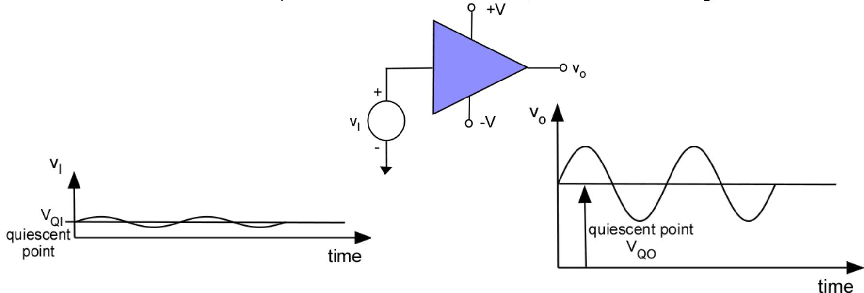
$$V_I(t) = V_{QI} + v_I(t)$$
