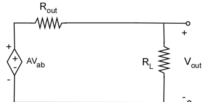
$$A_{MB} = \frac{V_{out}}{V_{in}} = \frac{R_{in}}{R_g + R_{in}} A \frac{R_L}{R_{out} + R_L}$$
