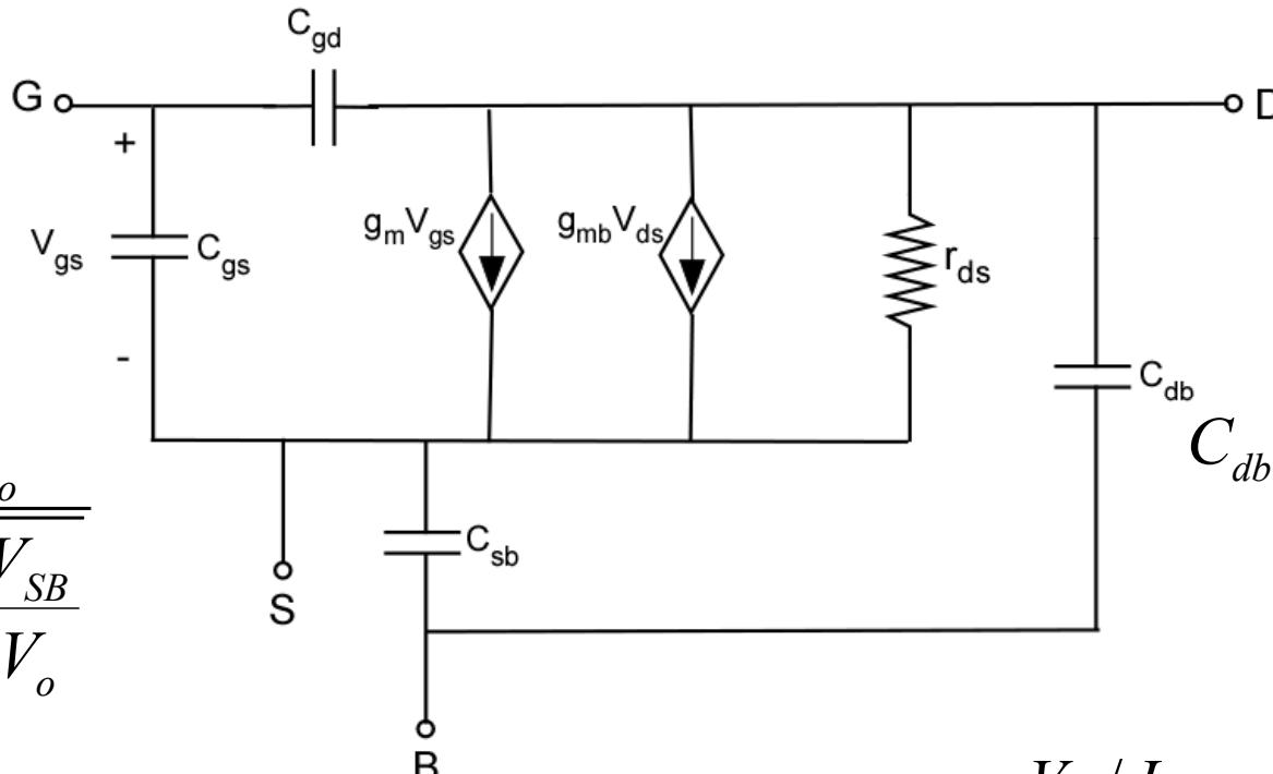
$$C_{sb} = \frac{C_{sbo}}{\sqrt{1 + \frac{V_{SB}}{V_o}}}$$
