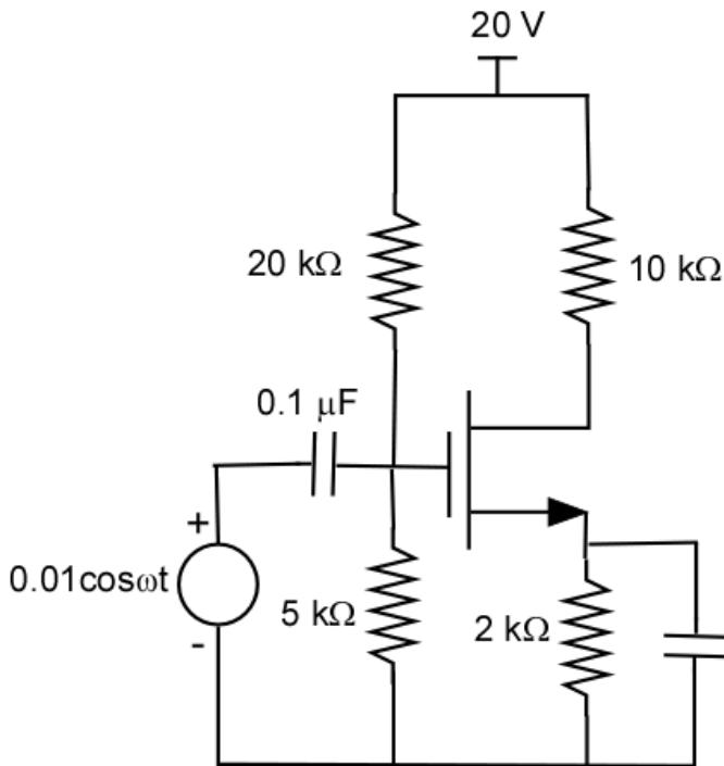
$$V_{GQ} = V_{DD} \frac{R_2}{R_1 + R_2} = \frac{20 \times 5}{25} = 4 \text{ V}$$
