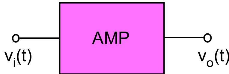
$$v_o(t) = A v_i(t), \text{ where } A \text{ is the voltage gain}$$
