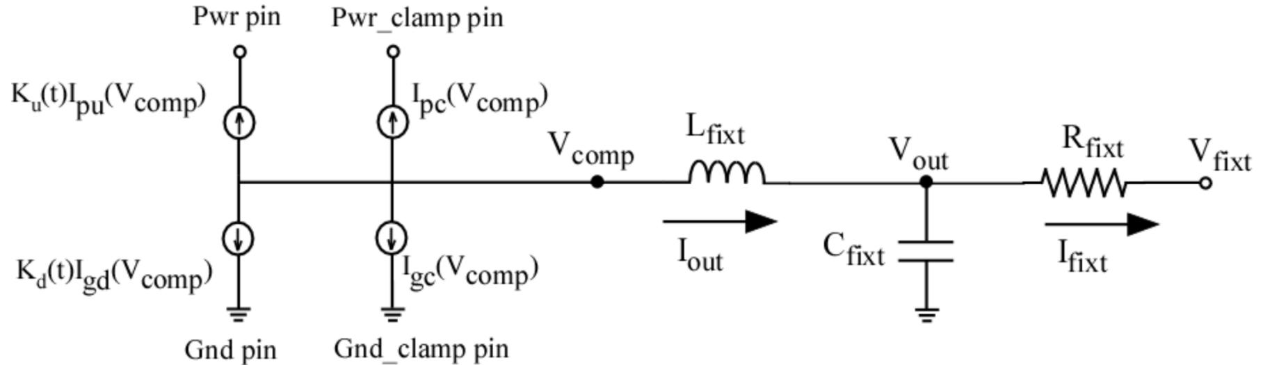
$$I_{fixt} = \frac{V_{out} - V_{fixt}}{R_{fixt}}$$
