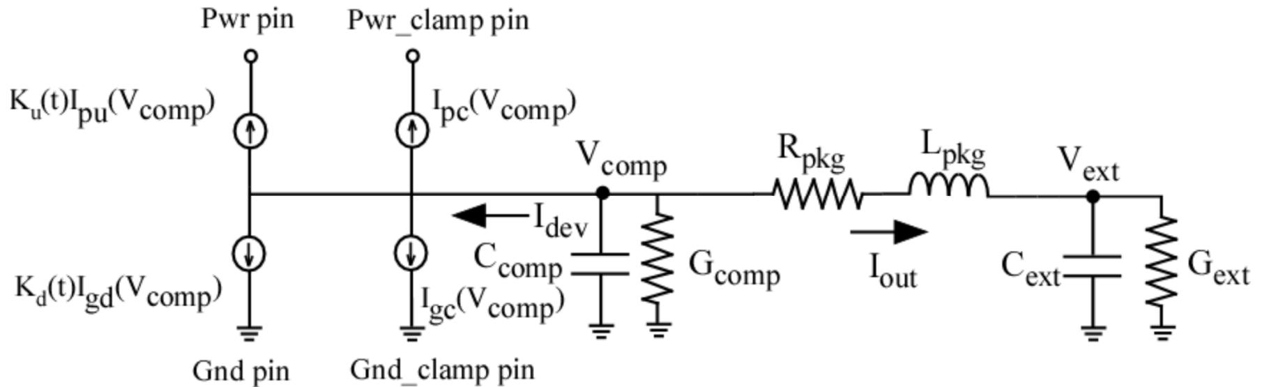
$$K_u I_{pu} (V_{comp}) + K_d I_{pd} (V_{comp}) + I_{pc} (V_{comp}) + I_{gc} (V_{comp})$$
