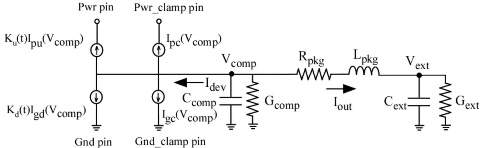
$$C_{ext} \frac{(V_{ext}^{n+1/2} - V_{ext}^{n-1/2})}{\Delta t} + \frac{G_{ext}}{2} (V_{ext}^{n+1/2} + V_{ext}^{n-1/2}) = I_{out}^n$$
