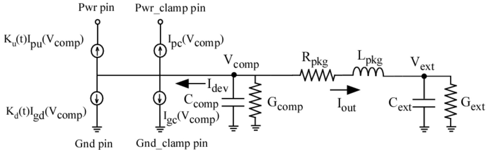
$$C_{comp} \frac{(V_{comp}^{n+1/2} - V_{comp}^{n-1/2})}{\Delta t} + \frac{G_{comp}}{2} (V_{comp}^{n+1/2} + V_{comp}^{n-1/2}) = -I_{out}^n - I_{dev}^n$$
