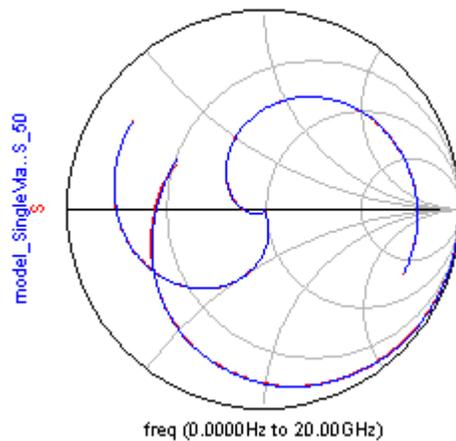
**Figure 14** Input and Output Comparison of S-Parameters using a Smith Chart Plot.
