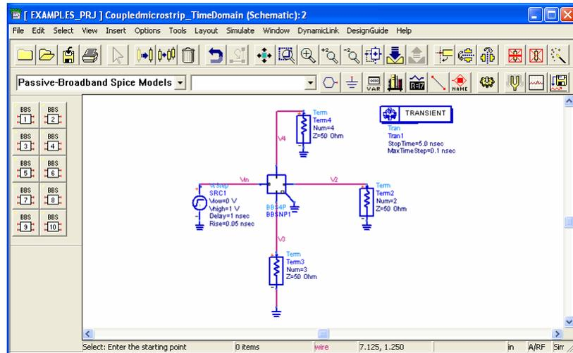
**Figure 18** Transient Simulation of the Broadband SPICE Component
