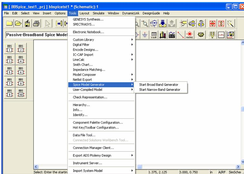
Figure 2 Starting the Broadband SPICE Model Generator.
