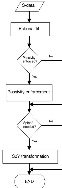
Figure 1 Broadband SPICE Model Generator Process Flow Chart
