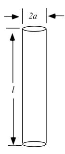
1. Write a program to calculate the charge distribution on a straight thin wire of length l and radius a (<< l), held at a potential 1V as shown above using the method of moments. Show a plot of the charge distribution for the case where l = 1 m and a = 1 mm.
