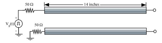
The pulse characteristics for  $V_g(t)$  are as shown in the figure below, with time delay:  $t_d = 1$  ns, rise time:  $t_r = 1$  ns, fall time:  $t_f = 1$  ns, pulse width:  $t_w = 20$  ns, pulse amplitude:  $V_{max} = 1$  volt
