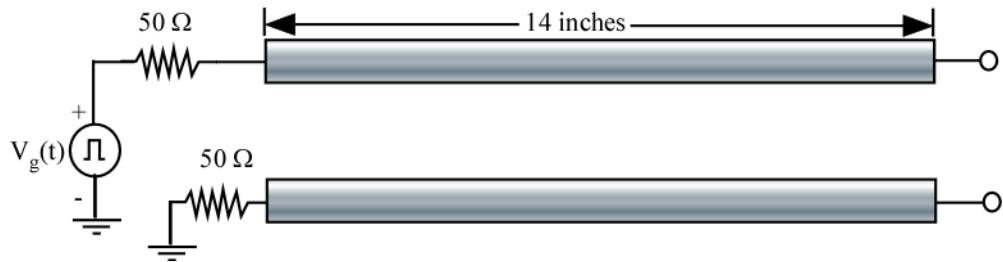
The pulse characteristics for  $V_g(t)$  are as shown in the figure below, with time delay:  $t_d = 1$  ns, rise time:  $t_r = 1$  ns, fall time:  $t_f = 1$  ns, pulse width:  $t_w = 20$  ns, pulse amplitude:  $V_{max} = 1$  volt
