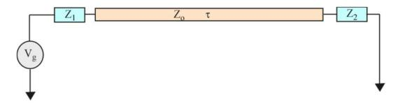
The pulse characteristics for  $V_g(t)$  are as shown in the figure below, with time delay:  $t_d = 5$  ns, rise time:  $t_r = 2$  ns, fall time:  $t_f = 2$  ns, pulse width:  $t_w = 20$  ns, pulse amplitude:  $V_{max} = 1$  volt
